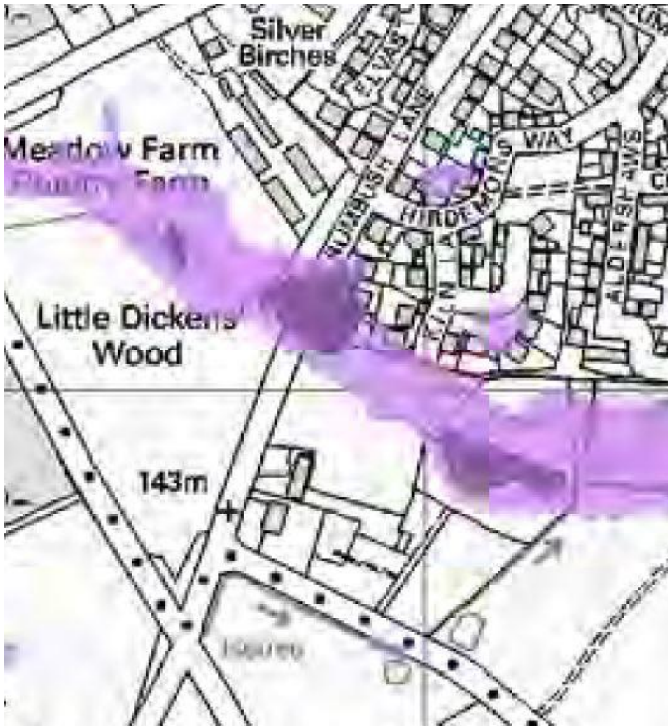
Fig 4: Environment Agency data showing flooding along line of existing brook
