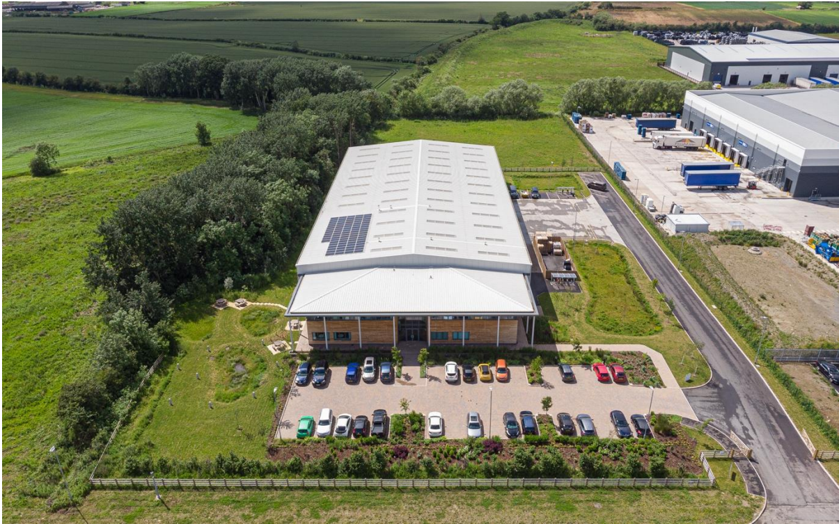
Building entrance showing the permeable parking area and rich vegetation to the building frontage associated with the raised wetland feature and linear raingarden.
