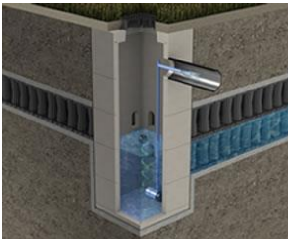
Figure 5 Subsurface attenuation installation and access chambers
