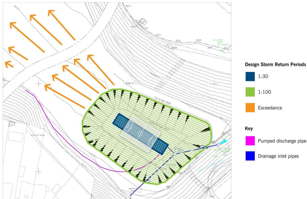
Figure 3 Runoff management integrating sub-surface attenuation and multi-functional elements such as the five-a-side sports pitch
