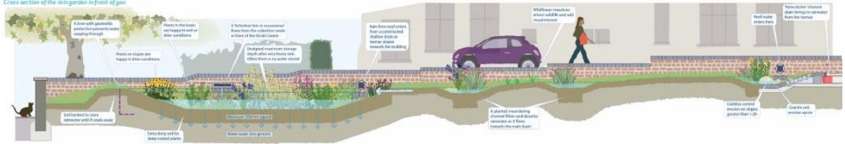
Cross section of the rain garden in front of gow
