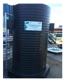
Fig 3: Hydrodynamic vortex seperator unit prior to installation
