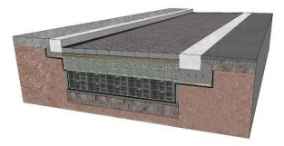
Figure 1: Cross section of permeable parking bay
