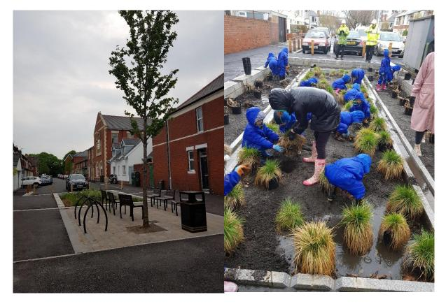
Figure 4 – Rain garden within regenerated public realm. Kerb and channel drainage keep water at the surface
