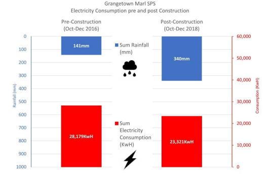
Figure 9 – Analysis of Rainfall in Cardiff and electricity consumption at Grangetown Marl SPS pre and post construction
