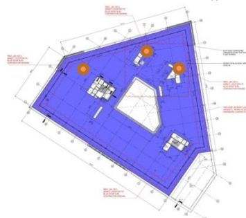
Level 60 bluroof extent showing the 4 restrictor chamber positions
