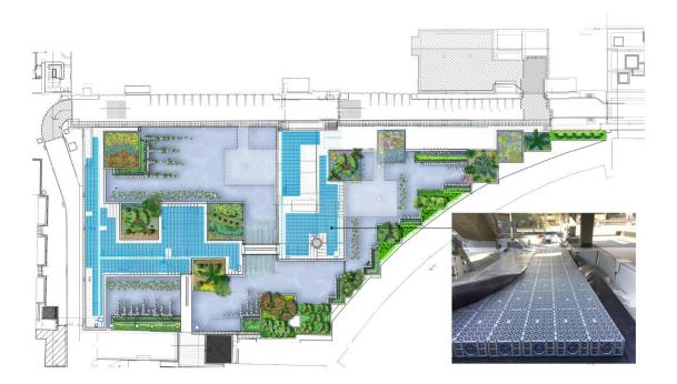
Fig 2. Rainwater geocellular storage and attenuation system on the podium deck.
