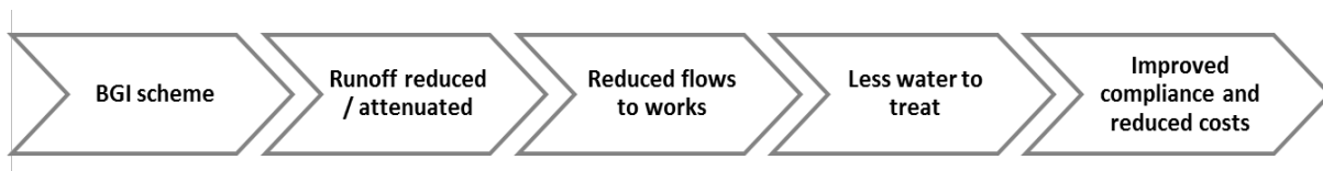
Figure 4-4 Impact pathway for wastewater treatment
