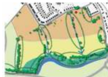
SuDS Opportunities and Constraints Diagram • High point • Low Point • Direction of flows • Flood risk zone • Biodiversity areas
