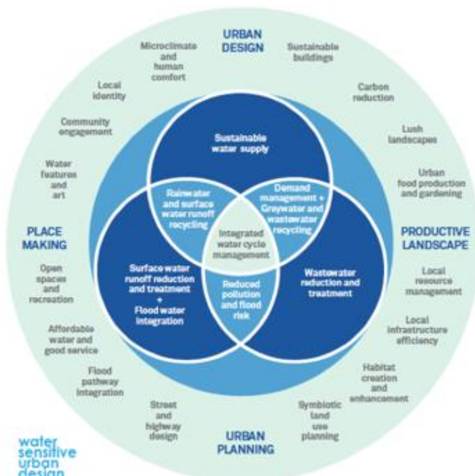
Figure 3.1 The linkages between the three streams of the urban water cycle, brought together in an integrated way that forms the WSUD process (CIRIA, 2013)
