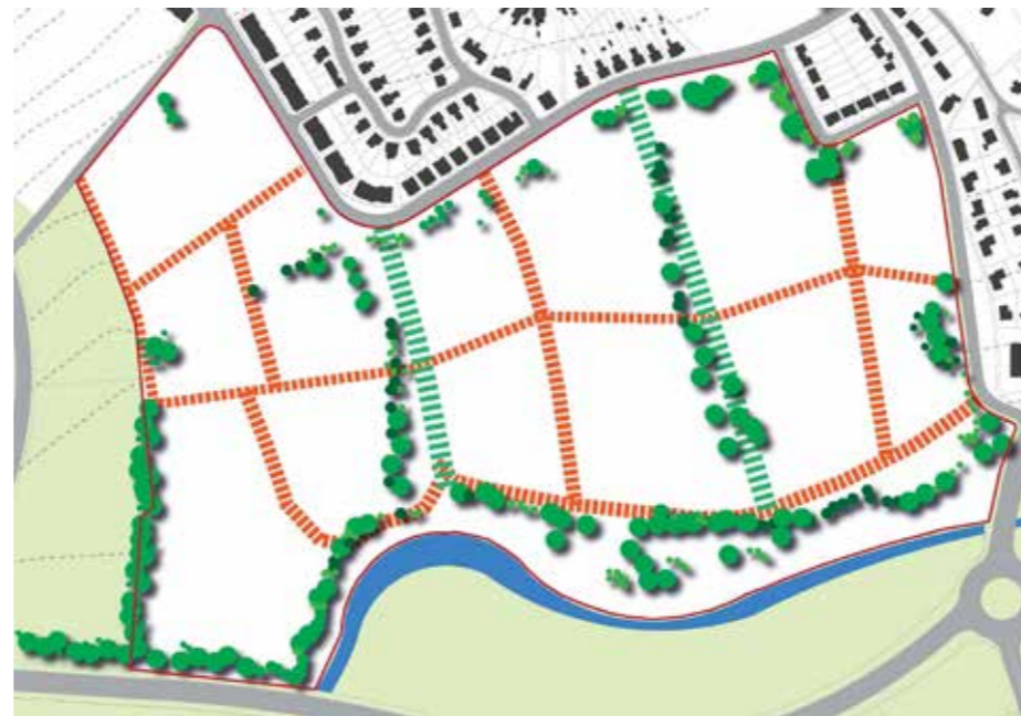
Street structuring for gravity surface drainage
