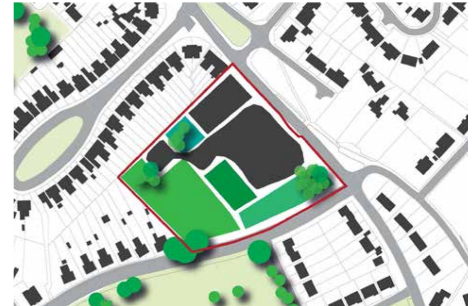
Impermeable and permeable space analysis
