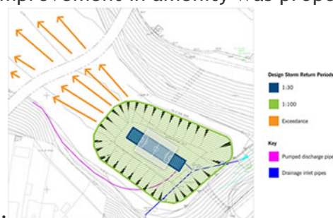
Figure 3. Runoff management integrating sub-surface attenuation and multi-functional elements such as the five-a-side sports pitch
